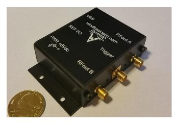
The SynthHD has powerful software and firmware features such as sweeps, lookup table frequency and amplitude hopping, pulse modulation, AM, FM and FMCW pulsed chirps. Experiment with dual super-het LO generation, quadrature LO generation, antenna beam steering and more. The SynthHD is a great addition to test equipment either in a lab environment or as a highly portable device used in the field. Also, the SynthHD works well as a basic building block in microwave communications systems.
