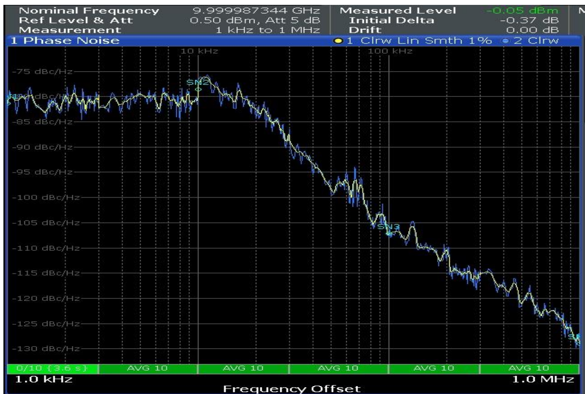
Typical phase noise at 10GHz
