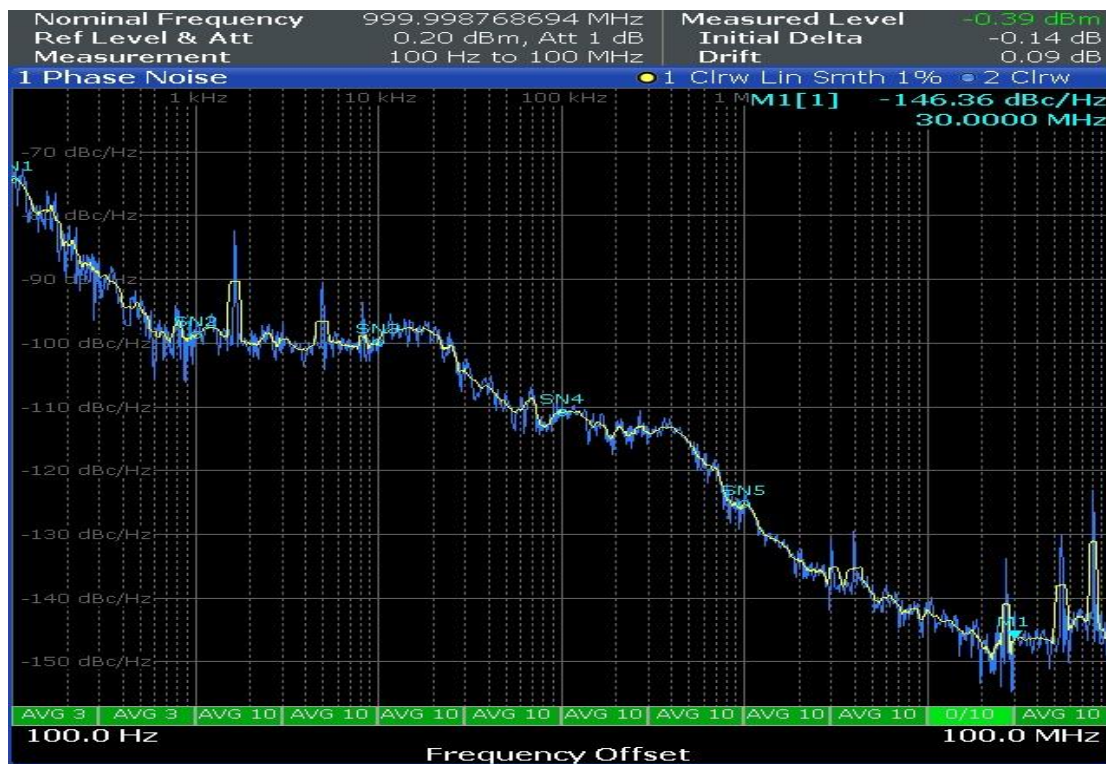
Typical phase noise at 1GHz
