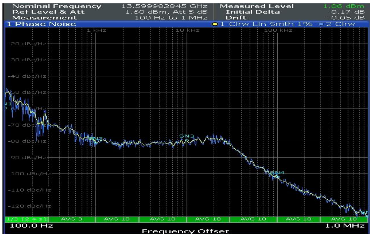
Typical phase noise at 13.6GHz
